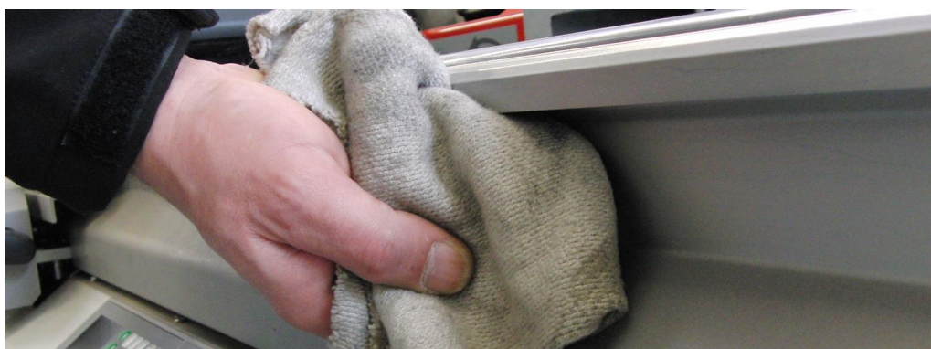
Fig. 8-2 Remove dirt from the bottom of the guide of the sliding table
