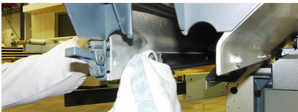
Fig. 8-3 Cleaning of the sub-rollers of the sliding table
